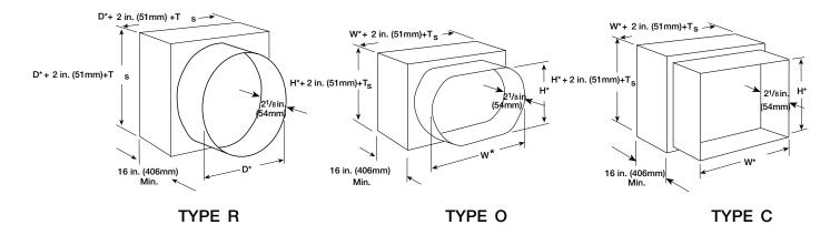
\* These dimensions are furnished approximately 1/4 in. (6mm) undersize, except round and oval dimensions which are approximately 1/8 in. (3mm) undersize. Ts = (2)(Sleeve Thickness)
